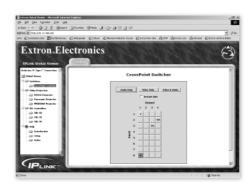
Example of screen to control an Extron CrossPoint matrix switcher.
